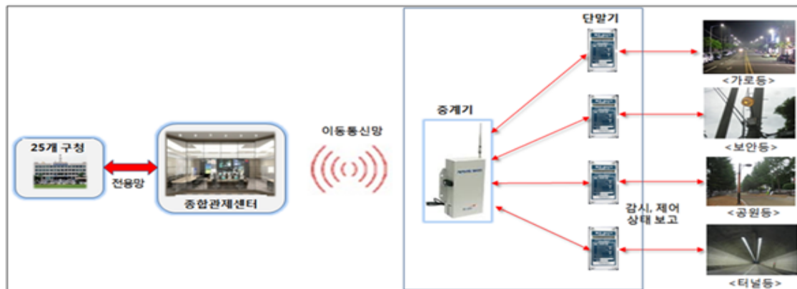
Figure 12. Diagram of smart lighting system
