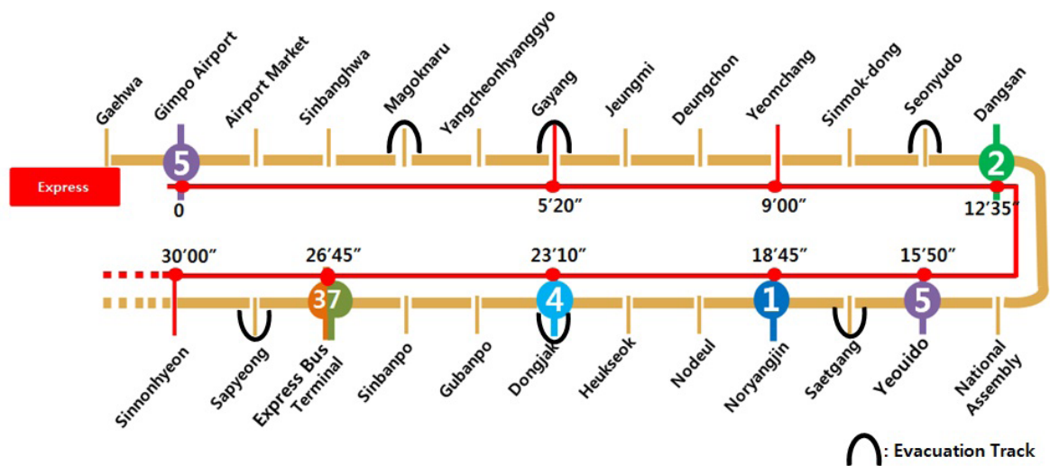
Figure 2 -Normal/ExpressTrains Operation Method in the Subway Line 9
